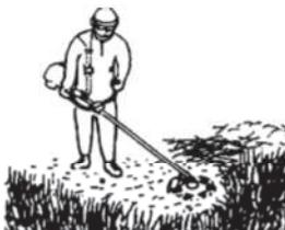
• Carry the machine to your right with the strap. Adjust the length of the strap to make the grass trimmer parallel to the ground.
