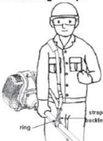
• Start the engine and keep it at idling. Wear straps as the following picture shows and buckle the pothook of the strap with the ring of bush cutter (grass trimmer).
