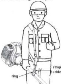
• Start the engine and keep it at idling. Wear straps as the following picture shows and buckle the pothook of the strap with the ring of the bush cutter (grass trimmer).
