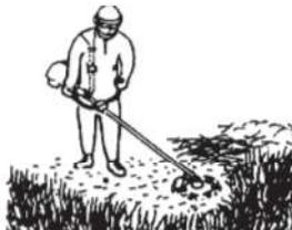
• Carry the machine to your right with the strap. Adjust the length of the strap to make the grass trimmer parallel to the ground.
